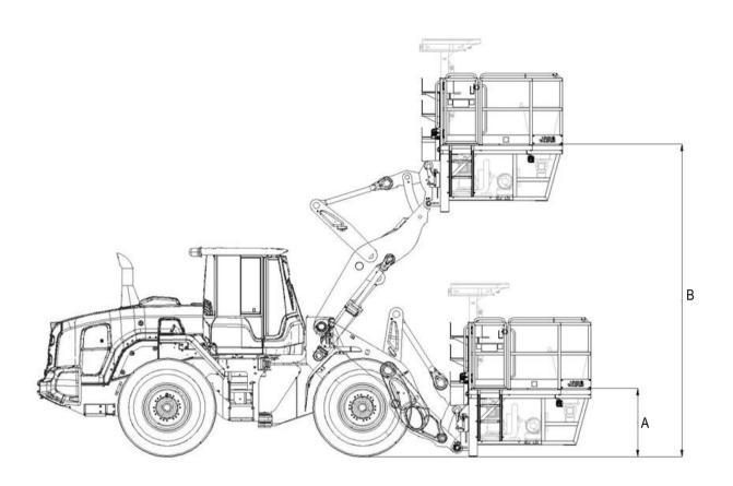
Mobile elevating working platform (MEWP) BK008 is together with Jama-modified versions Volvo wheel loader L70, L90 and L120\*, certified and approved for lifting persons. The platform can be operated either from the cabin or from the platform.
